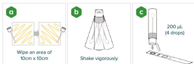
Fig 2. Test steps (a) Surface swabbing, (b) Sample preparation, (c) Application of test solution to Test Stick.
