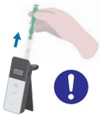
Be sure to remove the reagent after measurement. Failure to do so may lead to liquid leak.
